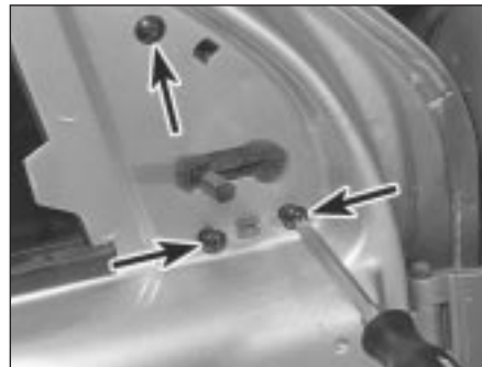
18.8 Removing the three mirror retaining screws (arrowed)
