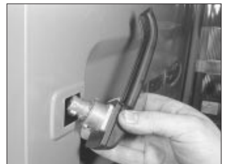
30.7b . . . to release Courier rear door exterior handle
