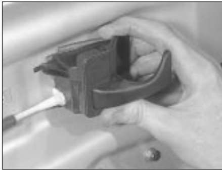
22.18 Detaching the interior door release handle
