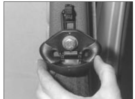
41.11 Removing a seat belt upper anchor cover
