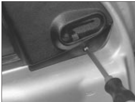
18.7 Removing the mirror trim retaining screw
