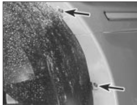
16.2 Front bumper-to-wheelarch retaining screws (arrowed)
