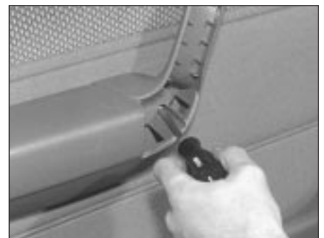
21.4b Undoing armrest/doorpull retaining screws
