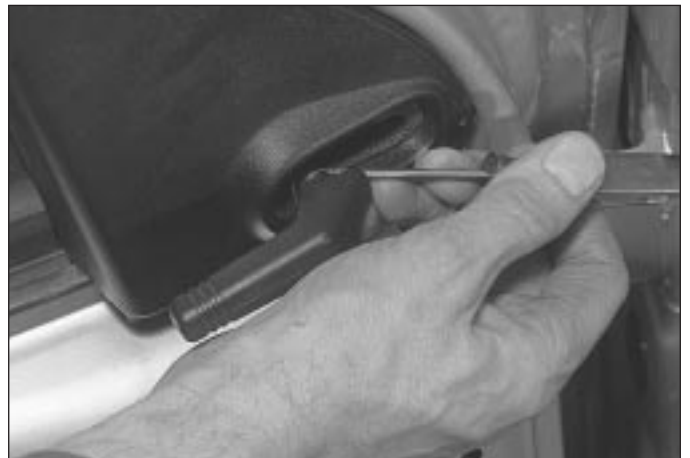
18.6 Lift the retaining clip, then pull the door mirror operating knob from its shaft
